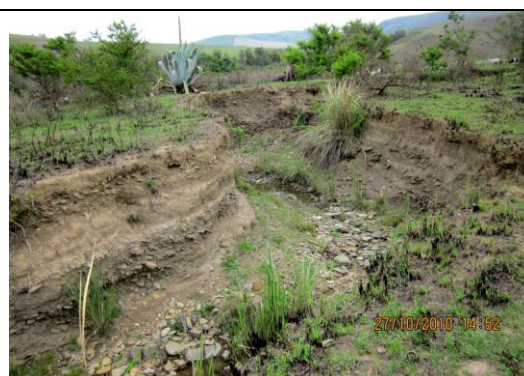
Plate 5. Alluvium upstream of centre line. Note sandy nature and gravel beds.
